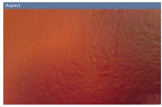
Rough or granular surface of the paint produced by bad stretching.
