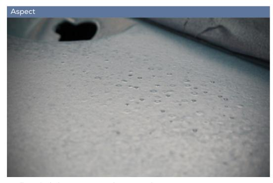
Small circular holes appearing on the paint surface.
