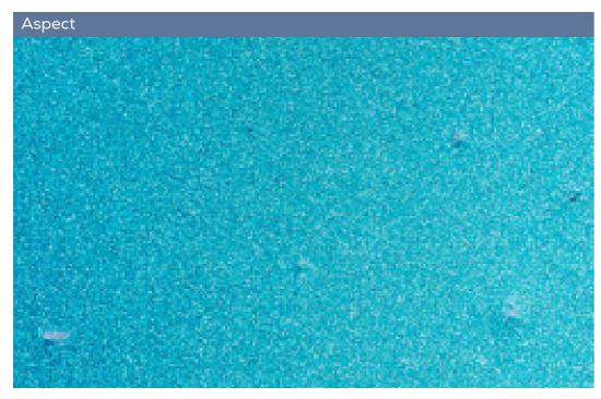
Dirt or dust depositing on the wet paint and sticking to it.
